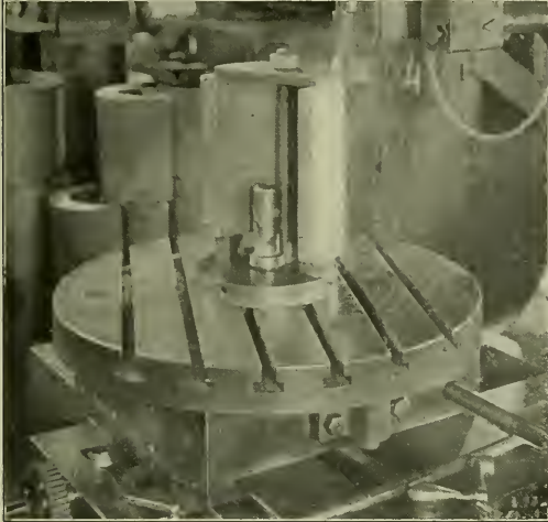
Fig. 1—Attachment for Slotting Driving Box Brasses.
